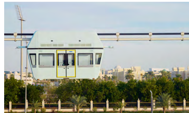
Electric Rolling Stock (uPods — unmanned rail electric vehicles on steel wheels)
